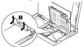
**Warning:** After replacing the hard disk drive, latch the removal strap into the correct position.
